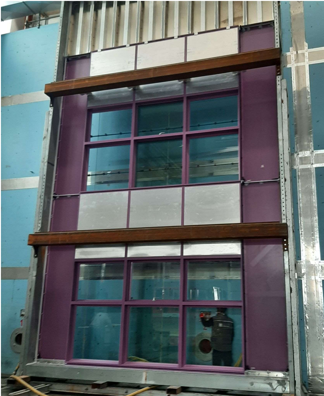
Figure 6 - PMU prototype installed and ready for the test
