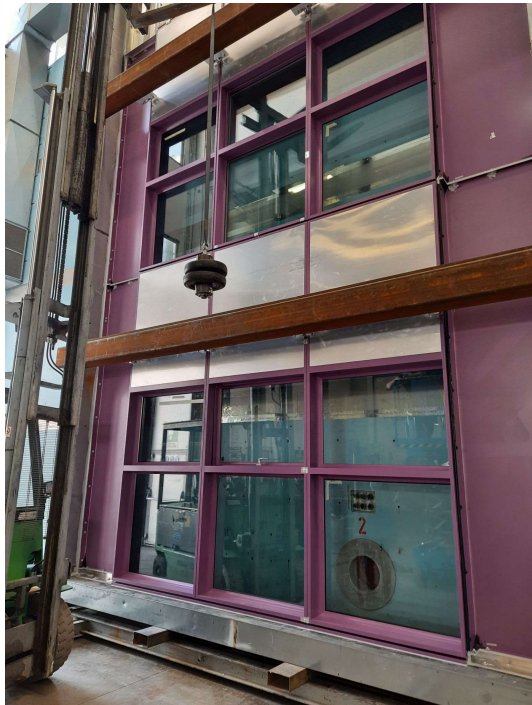
Figure 9 – Impact on the spandrel part top level in the metal sheet
