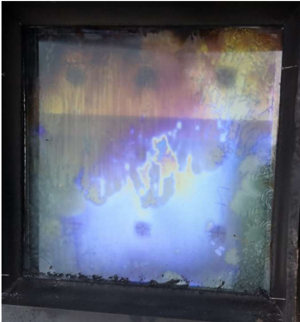
Figure 44 - Post test condition VIG-T3
