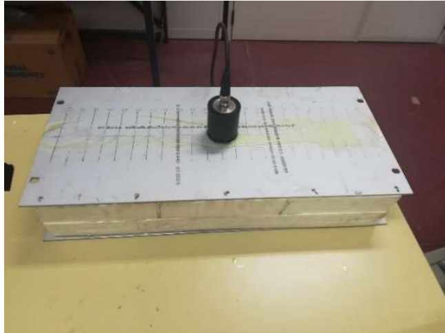
Figure 51 - The UT experimental set-up – Pulse echo mode.
