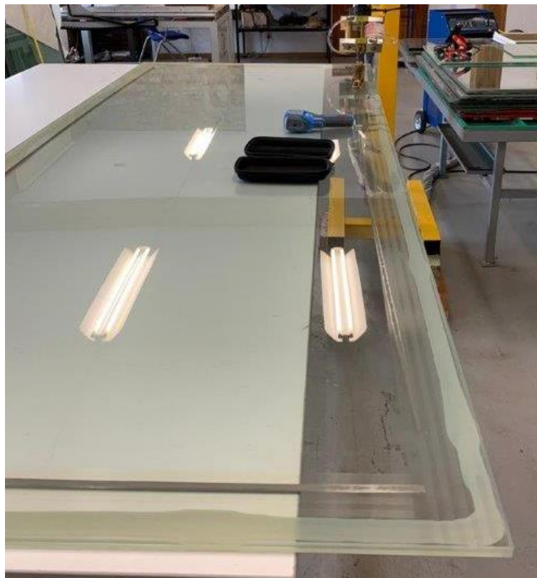
Figure 38 Vacuum glass preparation.
