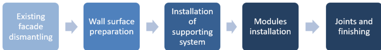
Figure 1 Work flow - Façade
