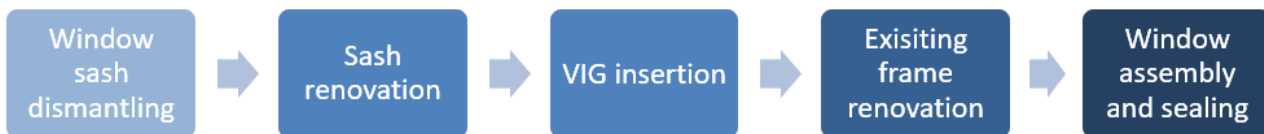
Figure 2 Work flow – Windows
