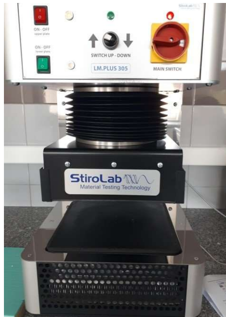
Figure 3-4 Thermal Conductivity test machine
