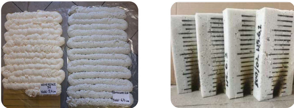
Figure 4-6 Developed OCF formulation compared with benchmark, B1– YIELD (left) and FLAMMABILITY CLASS (right)
