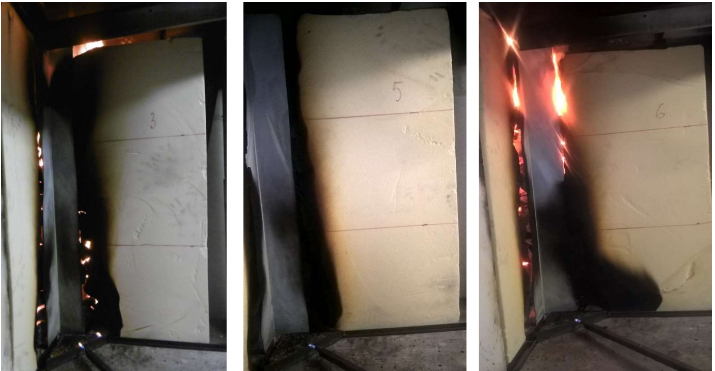
Figure 4-3 Pictures of tested samples after exposure to fire
