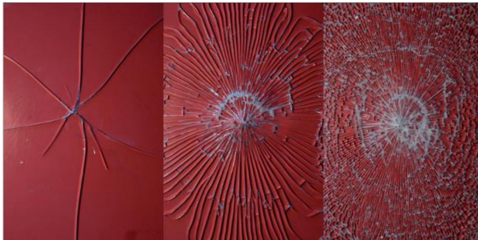
Figure 2-1 – Annealed glass failure (left), heat-strengthened glass failure (centre), and fully tempered glass failure (right).
