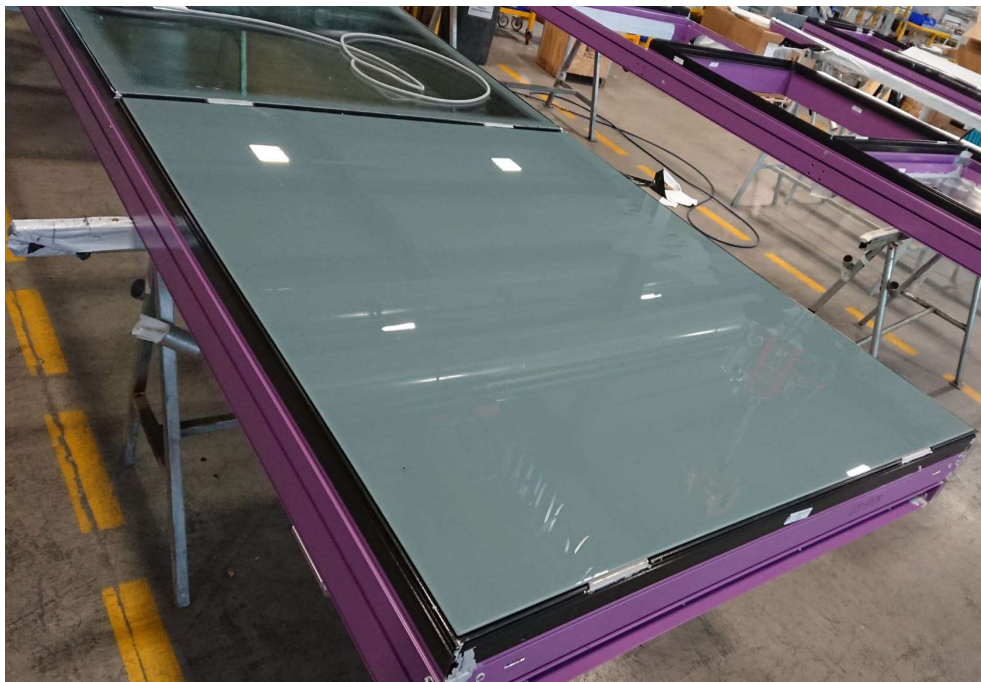
Figure 11 Spandrel part - glazing
