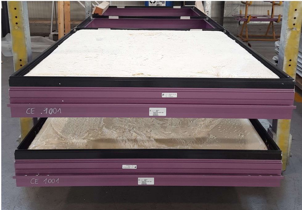
Figure 10 EENSULATE spandrel part ready to be glazed
