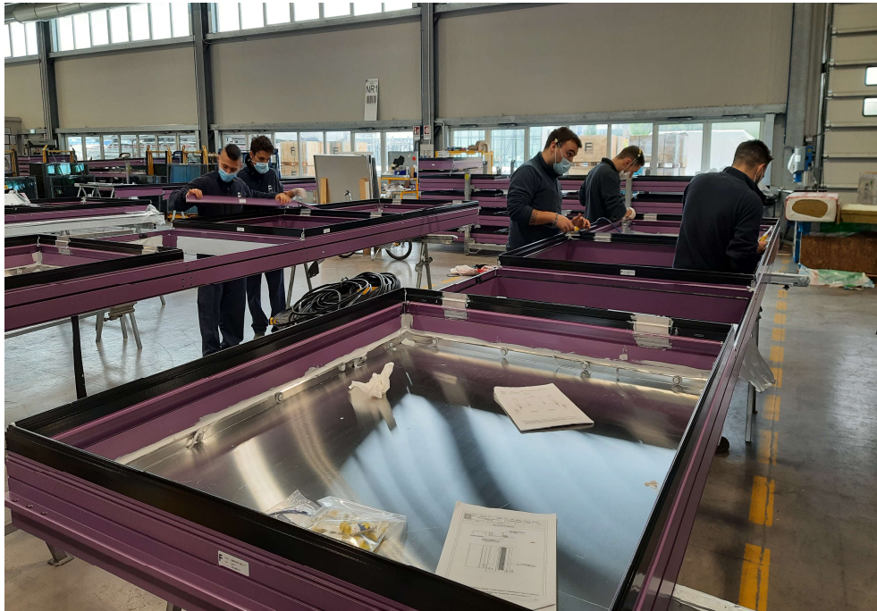
Figure 4 Spandrel part – metal sheet positioning
