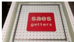
VIG small scale prototype after sealant curing
