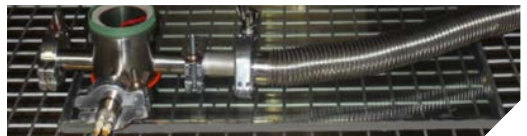
Pump down of sealed glazing
