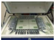
Pairing and clamping glass panes
